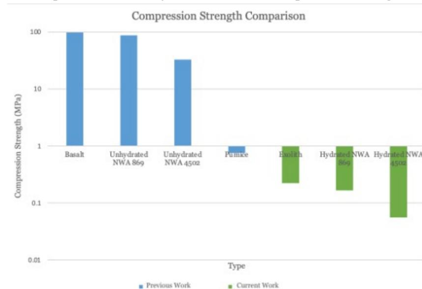
Figure 3. New compression strength tests on Exolith CC, Hydrated Northwest Africa 869, Hydrated Northwest Africa 4502, are compared with Pumice, Unhydrated Northwest Africa 869 [2], Basalt [4], and Unhydrated Northwest Africa 4502 [1] as performed previously in this lab.
