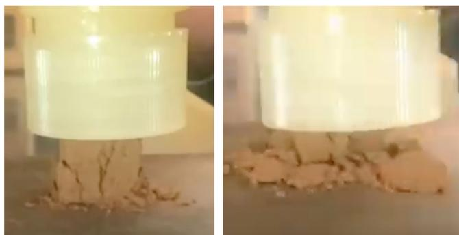
Figure 1. Close up images of the bottle method used to crush this sample of H-NWA 4502. The image on the left shows the first crack that occurred within the sample and the image on the right shows complete failure of the sample.
